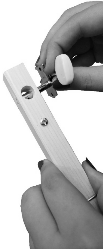
Figure 7 Insert tuning machine in side hole
