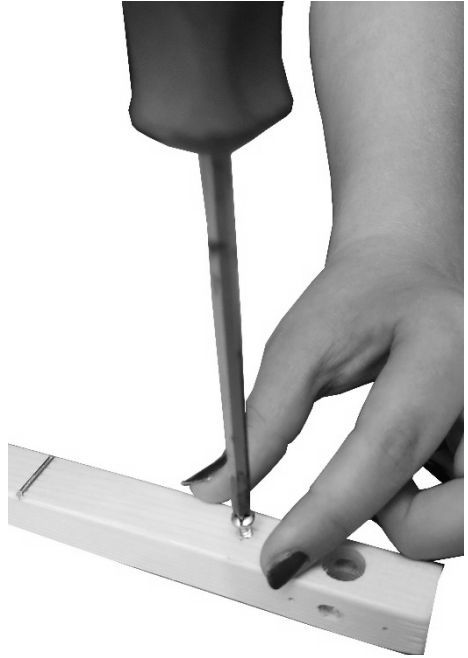
Figure 4 Installing the nut
