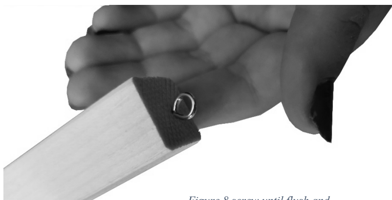
Figure 8 screw until flush and oriented properly
