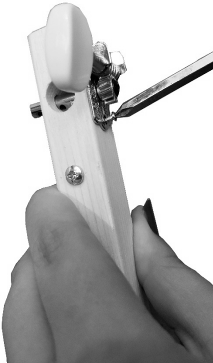
Figure 6 Install screws with Phillips #1
