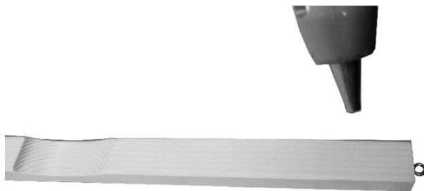
Figure 11 Applying the hot melt glue
